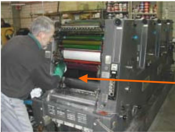
Permanent Press use a manual blanket wash system, which while slower than automatic systems it is claimed to use less solvent if properly undertaken.
