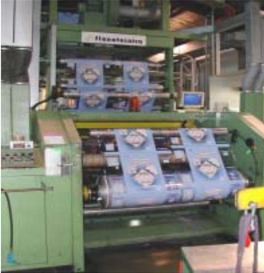
*This is one of Amcor's flexographic presses printing on polymer for food packaging – hygiene is very important on this site.*
