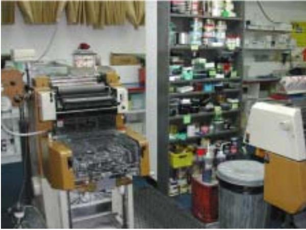
*The single colour lithographic printer resides next to its ink supplies. The printer was careful to store blended colours of inks from various clients. Being a single colour printer, individual colours have to be made up. This is in contrast to 4 colour printing machines, which can generate any colour from the basic 4.*
